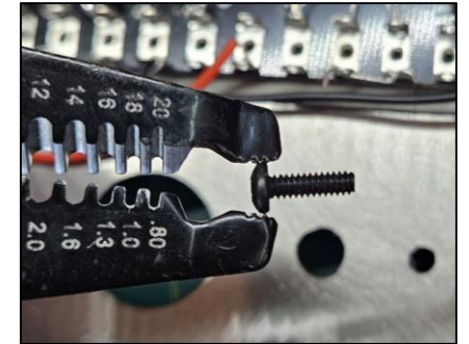
The tip of wire strippers have a jaw clamp to hold the bolts
