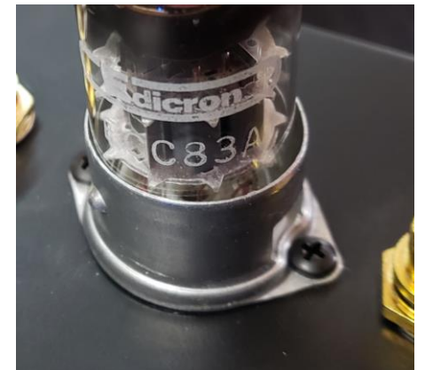
Bolts installed from the Outside, nuts on the Inside
