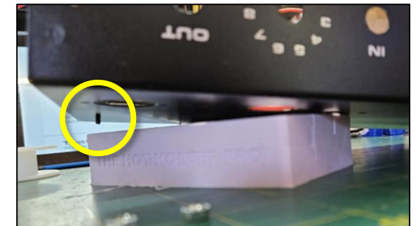
Raising the enclosure off the bench can help with bolt installation
